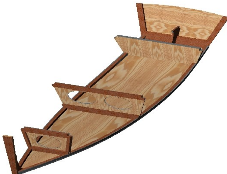
Fig.14. Bulkheads installation. The bulkheads are mounted to the floors on the keel laying with the help of epoxy glue and self tappers.
