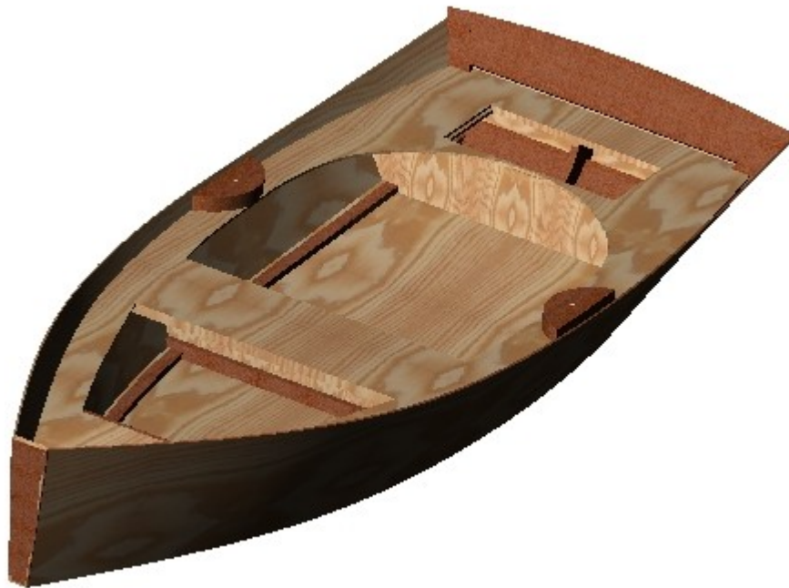
Fig.18.Side cover is fixed with help of glue and self tappers to bottom stringers and deck stringers.
