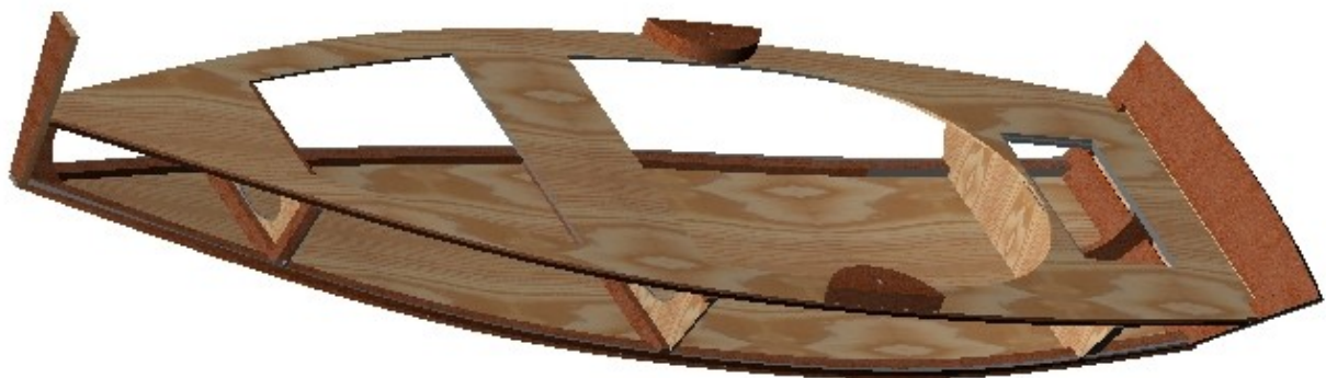
Fig.17. The board is mounted on the transom piece and rowlocks pillows. The distance between stern ward edge of the middle thwart and the rowlocks should be around 300 mm. Bottom stringers and deck stringers are beveled for side cover installation. Whether beveling is right can be checked by applying 400x1000mm plywood piece to the sides of the boat.
