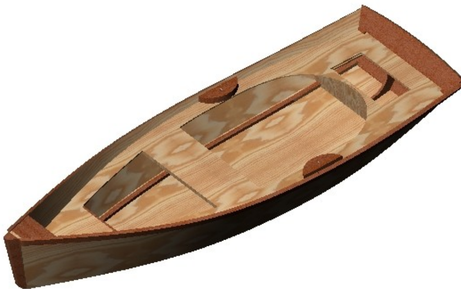
Fig.19. Keel laying is mounted on the stem (from the whole bar or 2 boards leftovers 25 mm). The strap is treated aflush together with the bottom and the sides. A slight rounding off is made from the side of the bottom. External clamps and rail cups are mounted.
